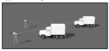
Two or more vehicles or buildings are connected by CableFree wireless products. Clear Line-of-Sight (LOS) for FSO or Near-Line-of-Sight (NLOS) for radio is required.
